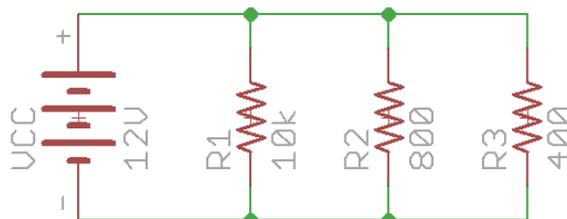
Figure 3: Parallel resistor circuit
