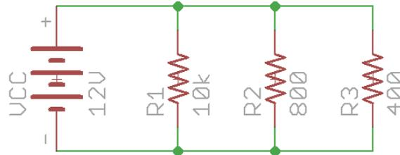
Figure 2: Parallel resistor circuit
