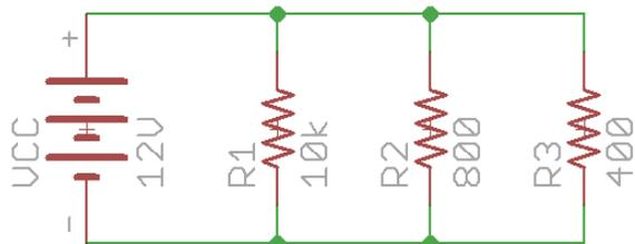
Figure 4: Parallel resistor circuit
